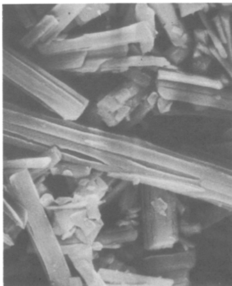
Picture 3 Scanning electron microscope picture of ulexite heated at 400^\circ C
